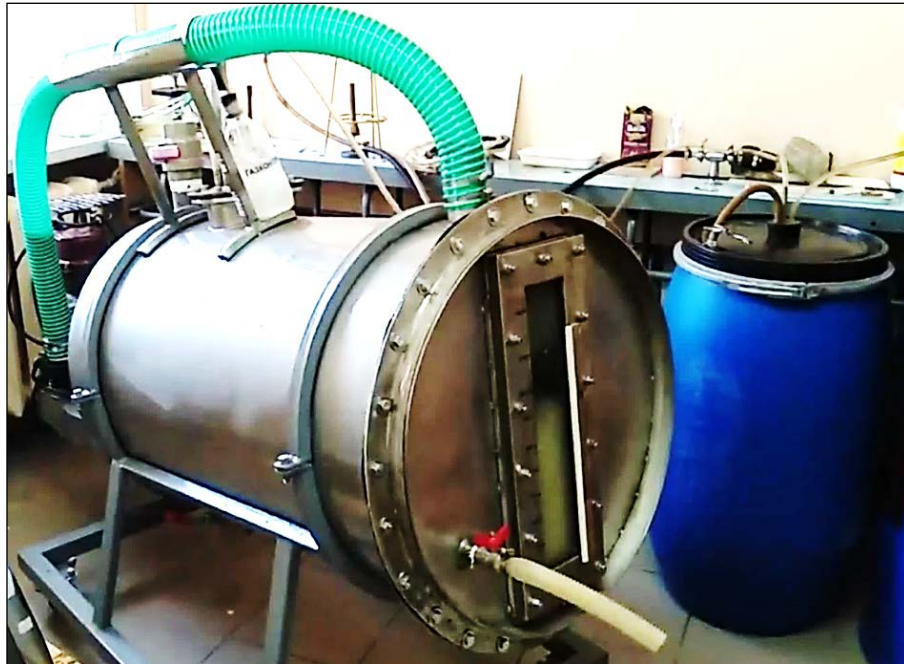
Picture 3. Biofermenter for fast and effective waste fermentation with an optimized design.
